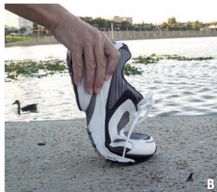
Figures 4 A, B: Forefoot flexional stability—Forefoot flexibility depends on both durometer of the midsole material and the depth of the flex grooves. Deeper grooves allow more flexibility of the shoe at the forefoot. The shoe should flex at the metatarsal-phalangeal joint, not further proximal through the midfoot.
