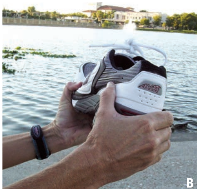
Figures 3 A, B: Midfoot torsional stability (shank rigidity)—Twist the shoe while grasping the heel and forefoot to determine the amount of stability or flexibility. Midfoot rigidity is necessary for running footwear.
