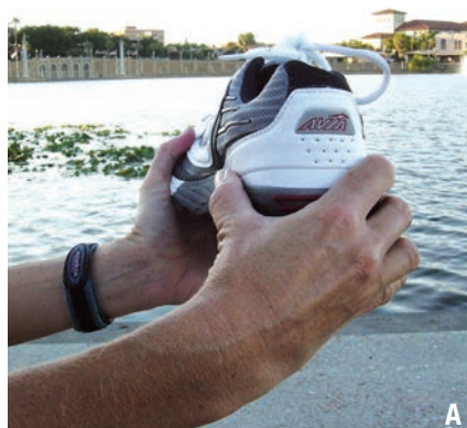
Figures 3 A, B: Midfoot torsional stability (shank rigidity)—Twist the shoe while grasping the heel and forefoot to determine the amount of stability or flexibility. Midfoot rigidity is necessary for running footwear.
