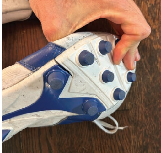
Figure 2 : Typical stress point on sole plate behind ball of foot
