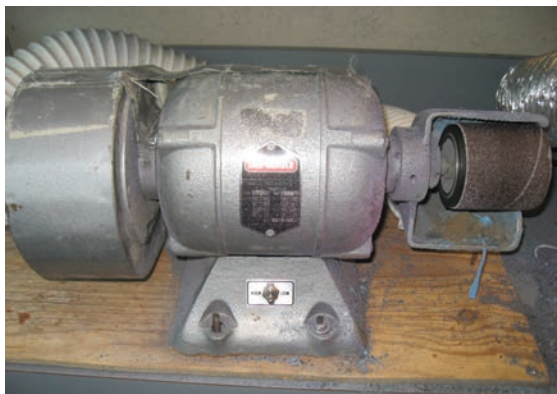
Figure 4: A grinder is an essential tool for orthotic practitioners. Among other uses, it can be used to thin the arch of the orthosis to increase flex and reduce reactive force applied to the plantar aspect of the foot.
