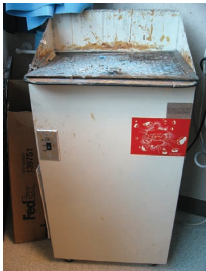
Figure 7: When working with glues, a hood or fume filter, such as this "Fume Buster" brand, are essential equipment. It functions as both a work surface and a fume filter.
