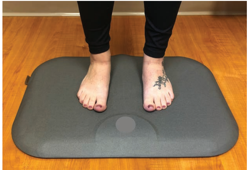
Figure 2: Utilization of a smart mat to provide temperature measurement of the foot
