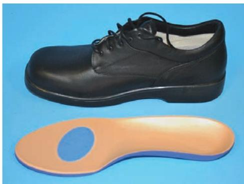
Figure 6: An extra-depth diabetic shoe with an insole fitted with a PTFE patch to reduce the coefficient of friction (COF) under the second, third, and fourth metatarsal heads, a common site of foot ulcerations in insensate patients. Photo courtesy of Strategic Medical Friction Management, Inc.
