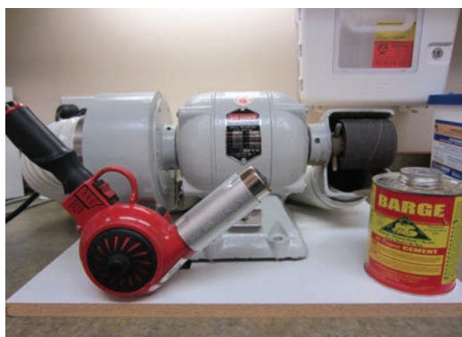
Figure 1: Orthotic modification equipment, including, from left: heat gun, grinding wheel, and glue.
