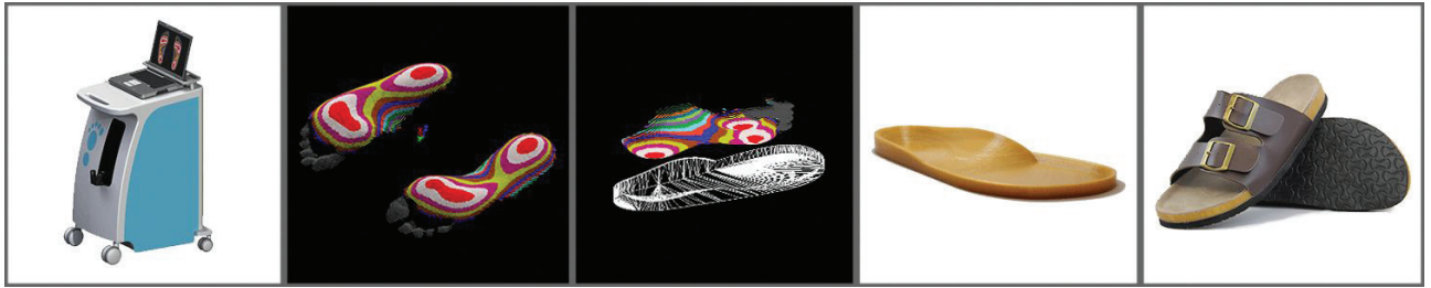
Figure 5: A sequence of customization for sandals. The feet are scanned, a digital model of the feet is created; next a digital model of the sandal foot bed is modelled and matched to a model of the foot and then printed. Finishing work involves laser-cutting a custom outsole, then gluing on a top cover, outsole, and straps. (Photo credit: OLT Footcare)
