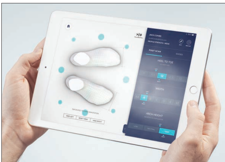
Figure 1: Volumental scanner relays the results of the scan to a tablet. It provides 9 measurements and ranked footwear recommendations based on a weight-bearing scan of the feet and can be used for customization as well. (Photo credit: Volumental)
