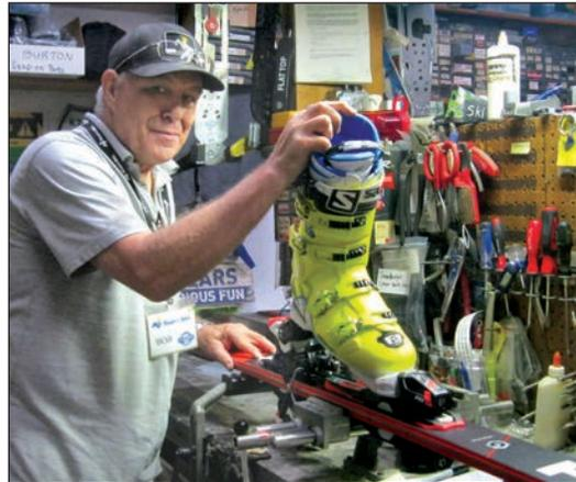
Figure 9: Custom boot fitter Bob, a Podiatrist, checking the boot and bindings for proper release
