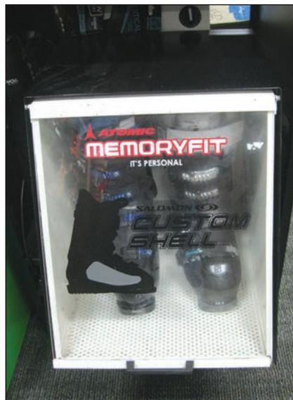
Figure 7: Heating machine to expand the outer shell for custom fitting
