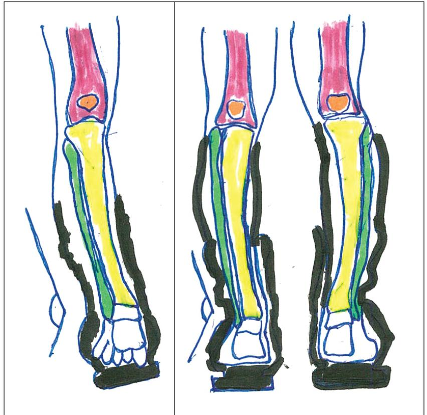
Figure 5: (Left) Uncompensated Tibia Vara in the Ski Boot: The boot cuff does not compensate adequately for the tibia vara, predisposing the skier to ride on the outside ski edge.
