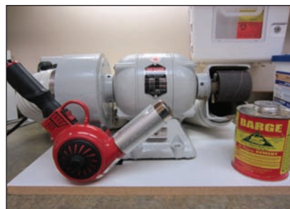
Figures 1: Orthotic modification equipment, including from left, heat gun, grinding wheel, and glue.
