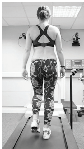
Figure 11: Sophisticated laboratory-based, multi-camera, computer-assisted VGA provides additional information but is still incapable of determining plantar pressure, path of pressure and accurate assessment of temporal parameters.
