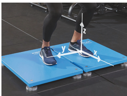
Figure 5: Subject standing on a force plate performing deep knee bends depicting the three force component pathways that are being measured. Note the elevation of the plates, causing “targeting” when conducting gait studies.
