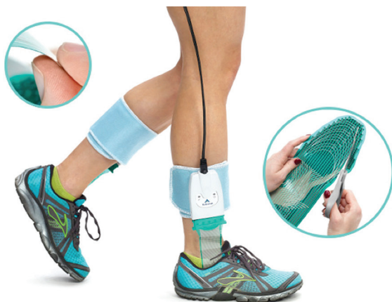
Figure 1: Thin, conformable, sensor imbedded insoles are trimmed to the subject's shoe and attached to an ankle connector
