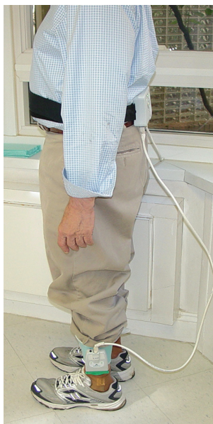
Figure 2: The cord from the ankle connector is attached to a small, unobtrusive, ergonomically designed waist pack recorder which is then remotely activated to begin a test
