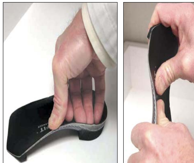
Figure 2 a,b: Non-compressible graphite composite device with flexural forgiveness and resistance to shell fracture.
