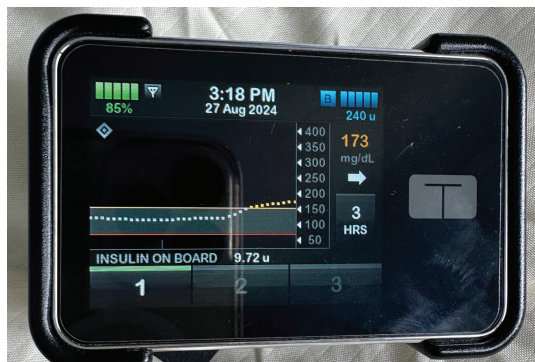
Figure 3c: The Dexcom G6 transmitter is also sending blood sugar information to the patient's Tandem T-Slim insulin pump to maximize blood sugar control.
