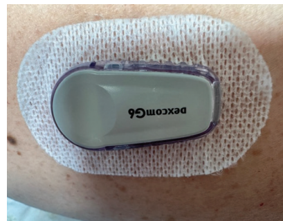
Figure 3a: A Dexcom G6 sensor is inserted into the skin testing the interstitial blood glucose on the patient's arm. A transmitter sending signals to a receiver or a cell phone to track the blood sugar trend. In addition, the transmitter can send signals to an insulin pump using a closed loop system to act like an artificial pancreas.
