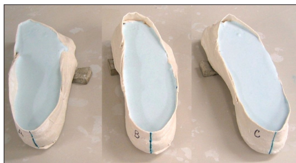
Figure 5: Wedges placed under forefoot areas of casts to align the heel vertical. Plaster of Paris is poured into negative casts
