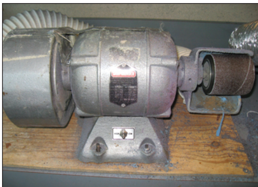
Figure 4: A grinder is an essential tool for orthotic practitioners. Among other uses, it can be used to thin the arch of the orthosis to increase flex and reduce reactive force applied to the plantar aspect of the foot.
