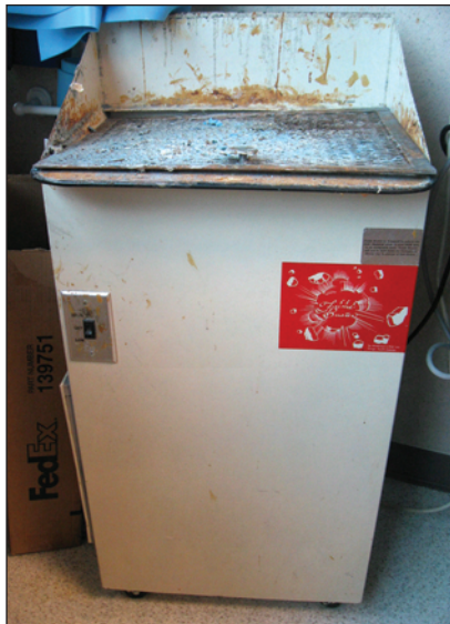
Figure 7: When working with glues, a hood or fume filter, such as this "Fume Buster" brand, are essential equipment. It functions as both a work surface and a fume filter.
