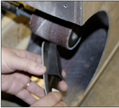
Figure 11: Grinding of the heel posts may be necessary to maximize shoe fit with the orthotic.
