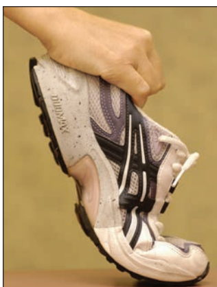
Figure 10, A and B: The flexion stability test is easily performed. Hold the heel of the shoe and press it into a flat surface at about 45-60 degrees. The shoe should bend at the ball of the foot (A). If it bends proximal to this point (B), it fails the test.
