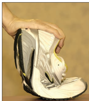
Figure 10, A and B: The flexion stability test is easily performed. Hold the heel of the shoe and press it into a flat surface at about 45-60 degrees. The shoe should bend at the ball of the foot (A). If it bends proximal to this point (B), it fails the test.
