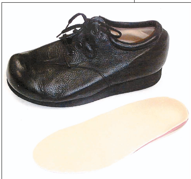
Figure 3: ExtradePTH shoe (P.W. Minor & Son, Batavia, NY) with enough room for insert. Shoe has blucher closure, wedge heel, stiff counter, and high wide toe box.
